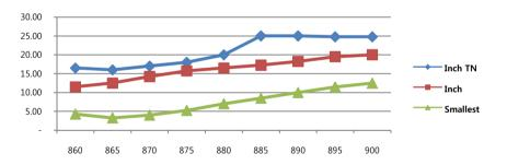
•INCH TN, second tiniest metal tag to NAIL, reads up to 0.7 meters on metal, 30% shorter than INCH (same size, but 1mm thicker than INCH TN). A few of similar size tags from other tag makers reads better, but none is as thin as INCH TN.
